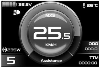
Press button in display 2 to enter display 3. In the riding condition, 5 seconds later, a single maximum speed (MXS) display automatically returns to the real riding speed (Km/H).
